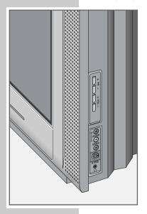
(1) Switches the television into and out of standby mode Channel selection PR -Switches the television on from standby + VOL -Adjusts the volume R AUDIO L Audio signal input for camcorder **VIDEO** Video signal input for camcorder S-VHS Video signal input for S-video camcorders Ω Headphone jack (3.5 mm ø jack plug)
